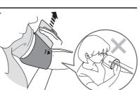
• When you take a measurement on the right arm, the air tube will be at the side of your elbow. Be careful not to rest your arm on
